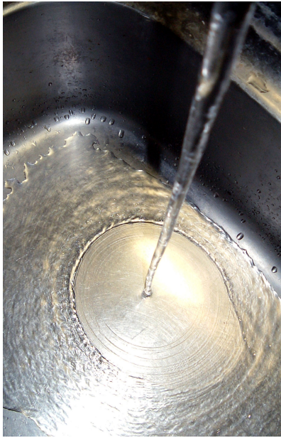
Figure 1: Hydraulic jump in a sink. By User Zeimusu on en.wikipedia - James Kilfiger took this picture, CC BY-SA 3.0.
